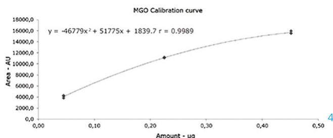
Calibration curve for quantification of MGO in Manuka honey samples
