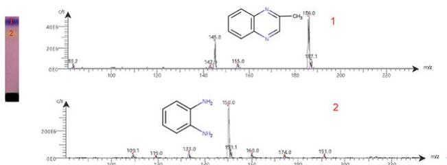
Mass spectra of 2-methylquinoxaline ( $m/z = 145.0$  [ $M+H^+$ ] and  $186.0$  [ $M+ACN+H^+$ ]) and 1,2-phenylenediamine ( $m/z = 150.0$  [ $M+ACN+H^+$ ])
