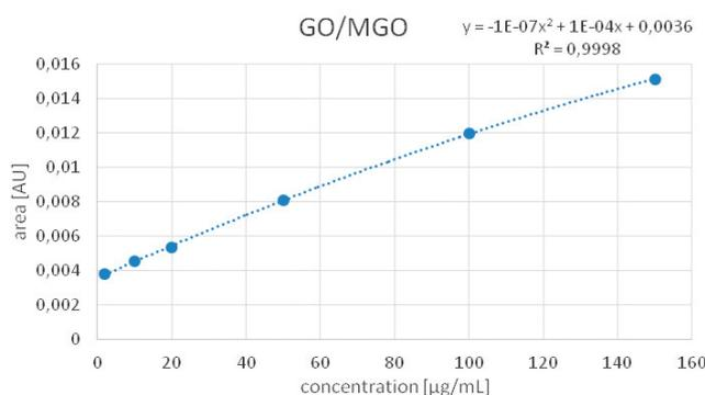
Calibration curve of GO/MGO at concentrations of 2–150  $\mu\text{g/mL}$  (measured in absorbance mode at 330 nm) [1]. (<https://creativecommons.org/licenses/by/4.0/legalcode>).
