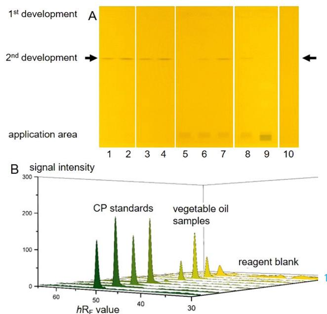
(A) Plate image after pSPE and derivatization with *o*-tolidine in white light and (B) corresponding 3D densitogram of the absorption scan at 645 nm of (1–4) from left to right, SCCP (chlorine content 55.5% and 63%), MCCP (chlorine content 52% and 57%), 225 ng CP/zone; (5–9) different vegetable oils, 7.5 mg sample/zone; (10) a reagent blank.
