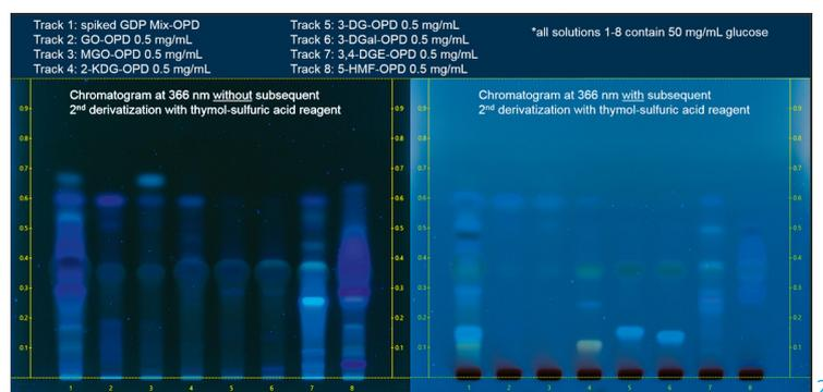
*Chromatograms of the derivatized seven GDPs and a mixture (= spiked glucose solution) in the solvent 1,4-dioxane – toluene – glacial acetic acid 49:49:2 (V/V). The chromatograms are shown in UV 366 nm without (left) and with (right) subsequent 2<sup>nd</sup> derivatization with thymol-sulfuric acid reagent at concentration levels of 0.5 mg/mL [1]. (<https://creativecommons.org/licenses/by/4.0/legalcode>).*
