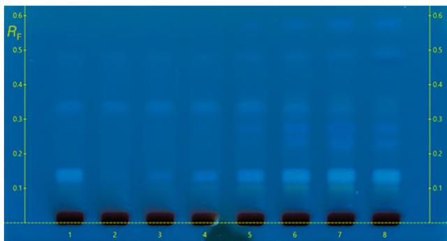
HPTLC chromatograms in UV 366 nm after both derivatizations (ROI until  $R_f$  0.6). Track 1 shows the spiked 5% glucose solution spiked GDP-Mix-OPD; tracks 2–8 the calibration solutions in ascending concentrations (1.0  $\mu\text{g/mL}$ –100.0  $\mu\text{g/mL}$  GDPs) [1]. All solutions contain 50 mg/mL glucose. (<https://creativecommons.org/licenses/by/4.0/legalcode>).
