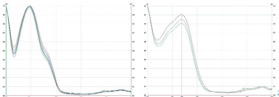
(Left) UV spectrum API no. 3 (red) and samples (cases no. 1–7); (right) UV spectrum API no. 2 (red) and samples (cases no. 8–9)
