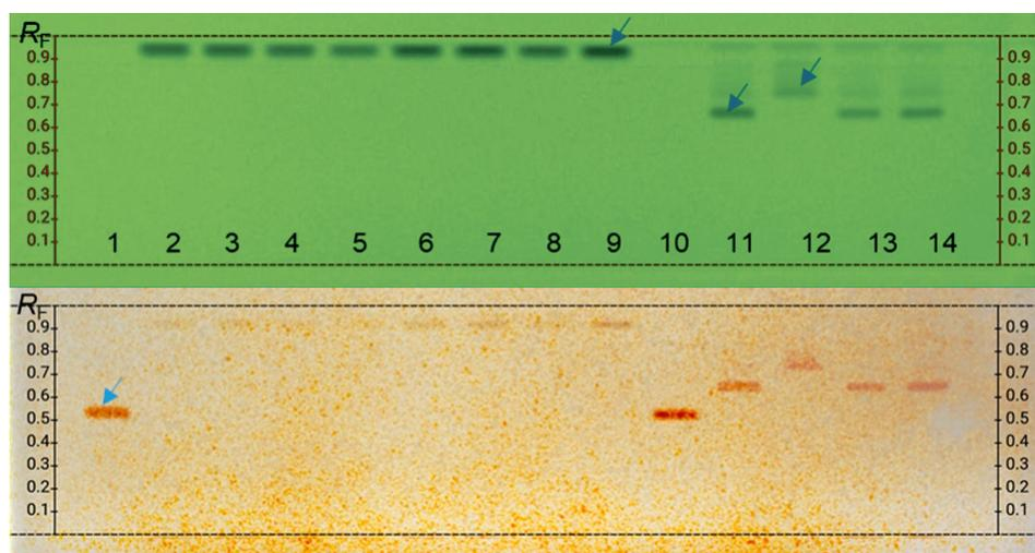
HPTLC chromatogram (top) in UV 254 nm prior to and (bottom) in white light after derivatization; tracks 1&10: API no. 1; tracks 2–8: cases no. 1–7; track 9: API no. 3; track 11: API no. 2; track 12: impurity of API no. 2; tracks 13–14: cases no. 8–9
