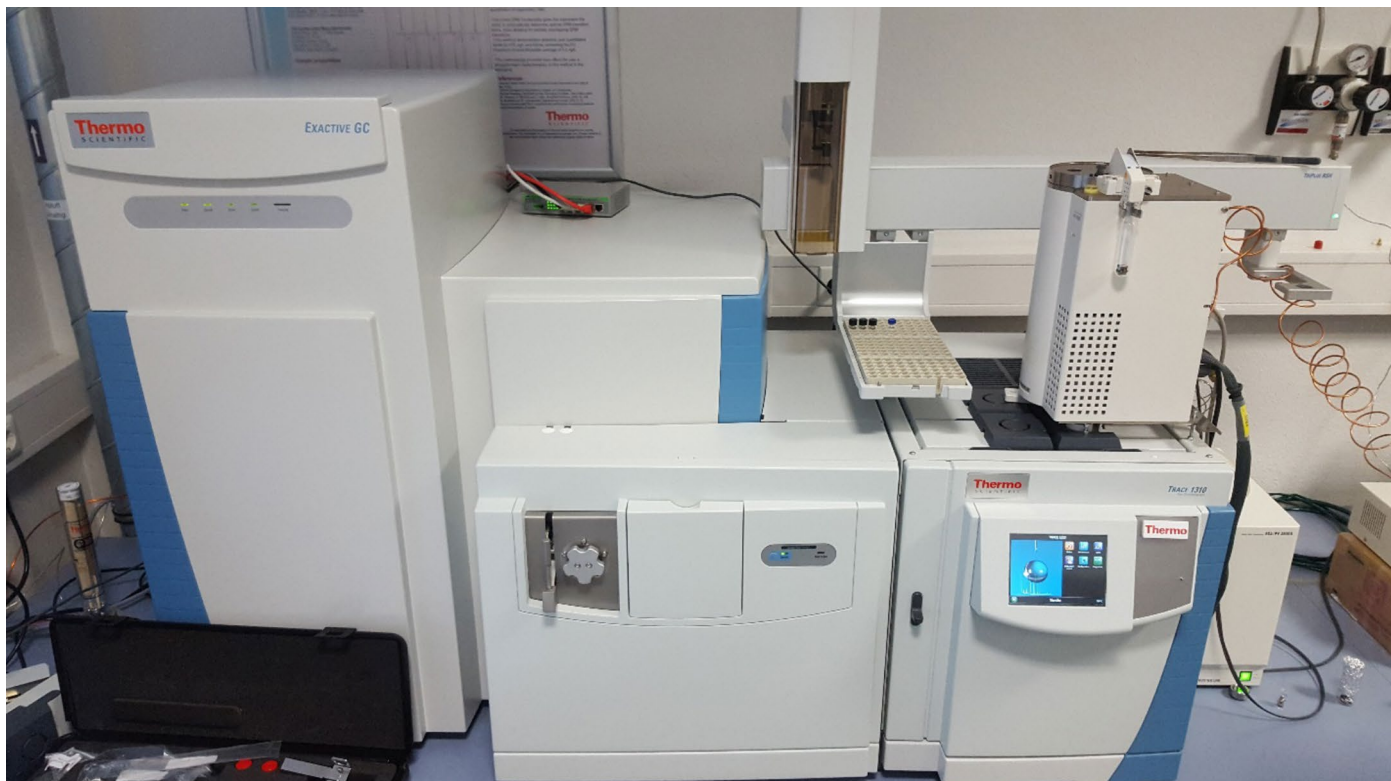
Figure 1. Instrumental setup: Multi-Shot Pyrolyzer (Frontier EGA/PY-3030D) with Auto-Shot Sampler (AS-1020E) coupled to an Exactive GC Orbitrap mass spectrometer
